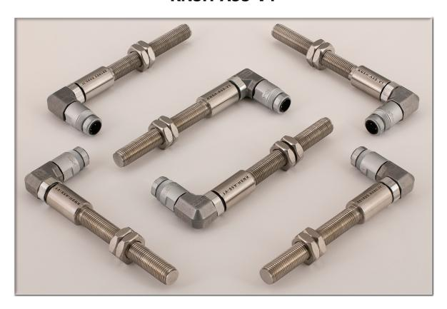
The KNSH-A5Sseries gear tooth speed sensors are Hall Effect devices designed for use in applications such as turbines, compressors, expanders etc.. Using a Hall-effect semiconductor device, the SH sensor detects the change in magnetic flux and converts this parameter into square-wave signals in the built-in electronic unit.
