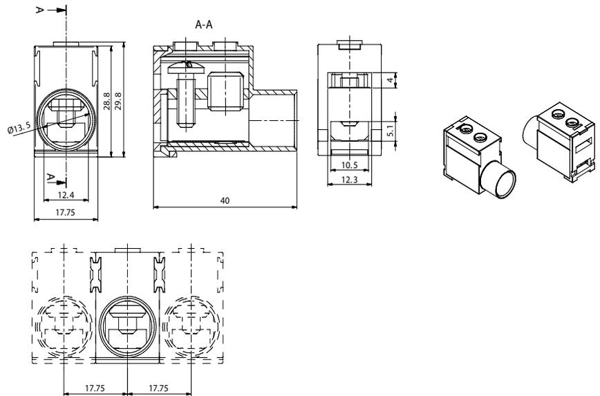
**Attention! Z-EK/35/UL supply terminals may only be installed per the illustration below.**
