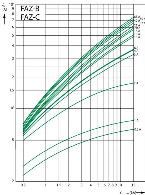
Circuit breakers that are classified as "current limiting" have the ability to clear damaging short circuit currents within the first half cycle of the fault, resulting in better overall protection for all circuit components.
