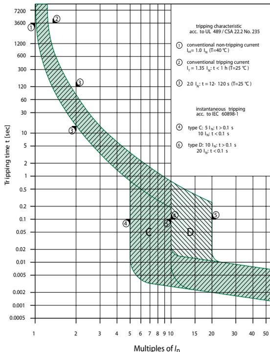
This graph shows trip-time versus over-current for Type C and D devices FAZ-NA branch circuit breakers.
